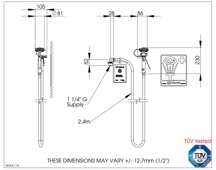
Free acces to the eye/facewash & body spray 8901RFK Axion must be guaranteed at all times. The operator is responsible for the observance of this requirement.
