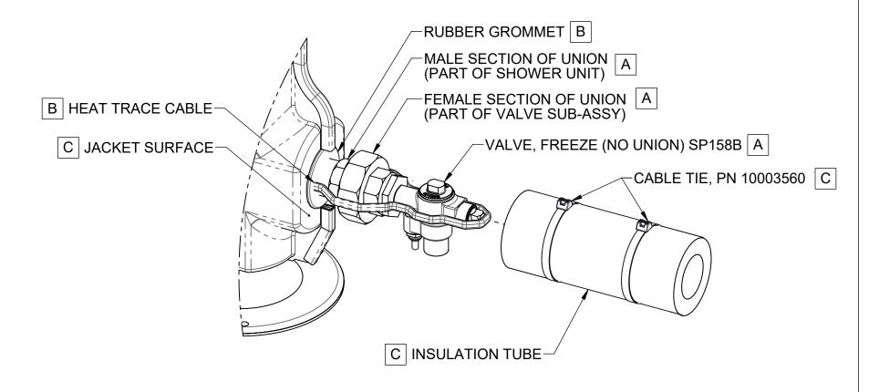
SP158B VALVE SHOWN CONNECTED TO BOTTOM UNION FOR REFERENCE ONLY. VALVE CAN BE INSTALLED AT TOP OR BOTTOM.
