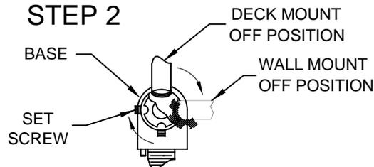
NOTE DEPTH OF SET SCREW PRIOR TO LOOSENING. LOOSEN SET SCREW AND ROTATE EYEWASH ARM 90° CLOCKWISE (AS SHOWN) WHILE MAKING SURE TO NOT ROTATE THE SPOOL. RE-TIGHTEN SET SCREW IN NEW POSITION. ENSURE SET SCREW IS PROPERLY SEATED IN INDENT. ENSURE SET SCREW IS TIGHT AND AT IT'S ORIGINAL DEPTH. ENSURE CORRECT ARM ORIENTATION BEFORE MOUNTING TO WALL. REFERENCE DRAWINGS AT RIGHT.
