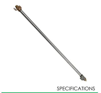
Model MK81A is a special freeze-protected valve that drains water from Model 8300FP combination shower/eyewash after closing to prevent freezing. 1-1/4" MIPS inlet. Standard sizes are 60" and 78" (152.4 and 198.1 cm) for bury depths of 24" and 42" (61 and 106.7 cm) respectively. Servicing Instructions: For replacement of damaged parts, order the VRKMK81A repair kit which includes packing, stuffing box, stuffing box nut, spring and plunger assembly with four O-rings.
