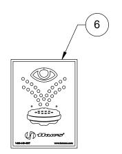
1 SP65 EYE/FACE WASH ASSEMBLY (INCLUDES: EYE/FACE WASH HEAD, ADAPTER, FLOW CONTROL, DUST COVER)
